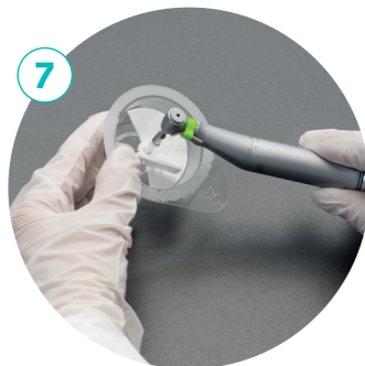
7 Attaching the contra-angle adapter or ratchet adapter by applying pressure
